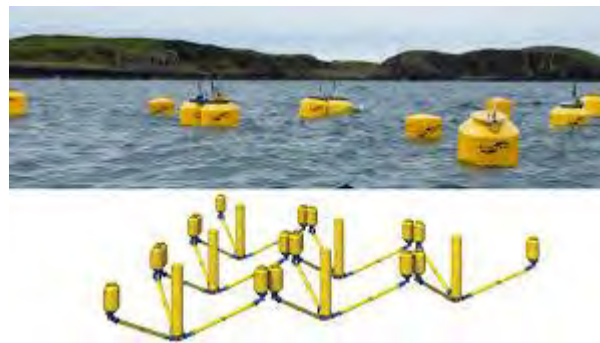
Figure 3.1: WaveNET 6S Array off the Isle of Muck, Scotland and SQUID Series-6 Generating Unit
